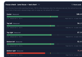
Focus check: reference 100 %, lower limit 85 %, only the bottom right is low (synthetic test chart, 0.1.0.23)
